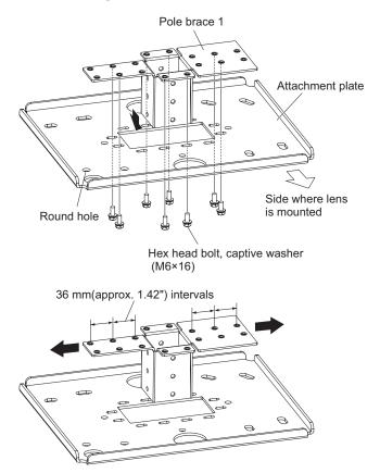
Insert the pole brace 1 into the center of the attachment plate, and secure the pole brace 1 with the supplied eight captive washer hex head bolts (M6  $\times$  16). (Refer to the figure on the left for the directions of the attachment plate and the pole brace 1.)
